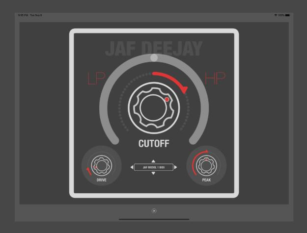
This Audio Unit, a filter unit, part of our JAF Series, is specialized for continuously fading the processed audio signal seamlessly between lowpass and highpass in performance situations. The center position of the cutoff will pass thru the unfiltered sound. A tube like saturation effect can be applied too.
